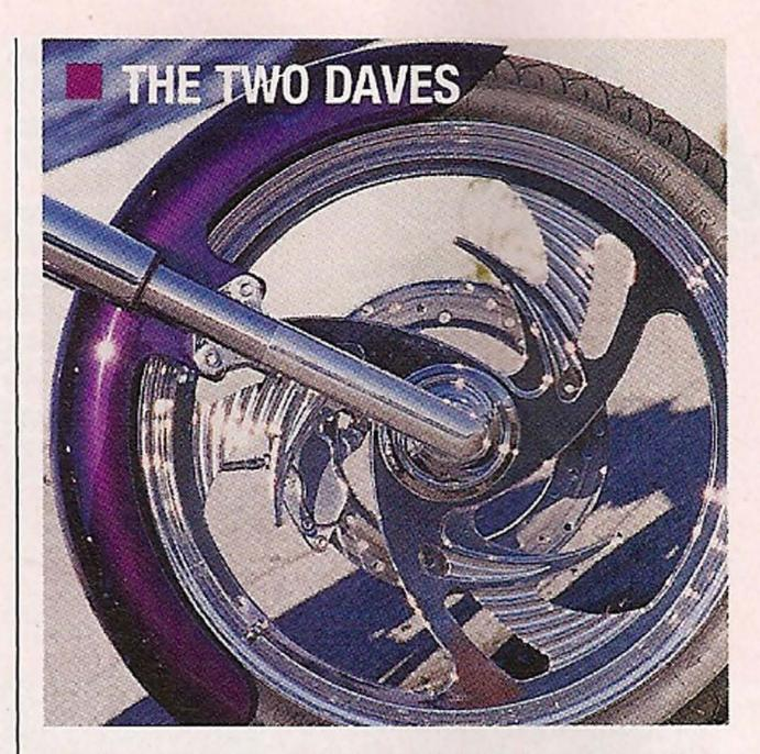
and a 200 tire for the 18x5.5-inch wheel at the rear. Matching rotors with P.M. calipers make for a brake system with sharp looks and excellent stopping power.
